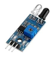
IR Sensor (Infrared Sensor): An IR sensor detects infrared light, allowing it to sense the presence or motion of objects. It's commonly used for proximity sensing or object detection in robots.
