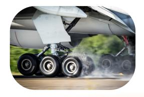
Aircraft Landing Gear: Hydraulic actuators are used to raise and lower the landing gear of airplanes during takeoff and landing.
